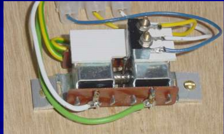
Simple microswitch mounting on a Peco solenoid
