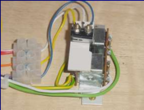
Simple microswitch mounting on a Peco solenoid
